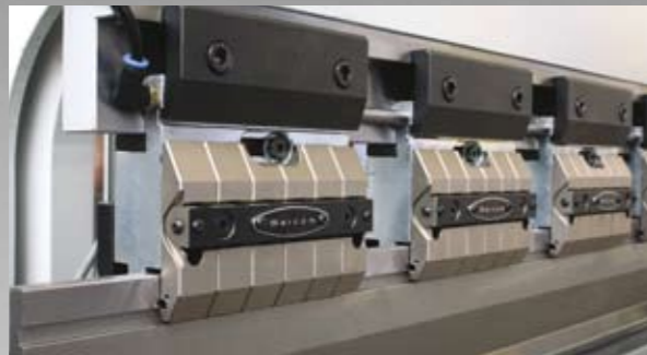
🇮🇹 Bloccaggio pneumatico mod. WTC ad inserimento frontale. Attacco promecam (senza fresature aggiuntive). Doppio reversibile. 🇬🇧 New WTC pneumatic clamping system with front insertion, European style hook (promecam), no additional grooves required. Available also in reversible version (front and rear).
